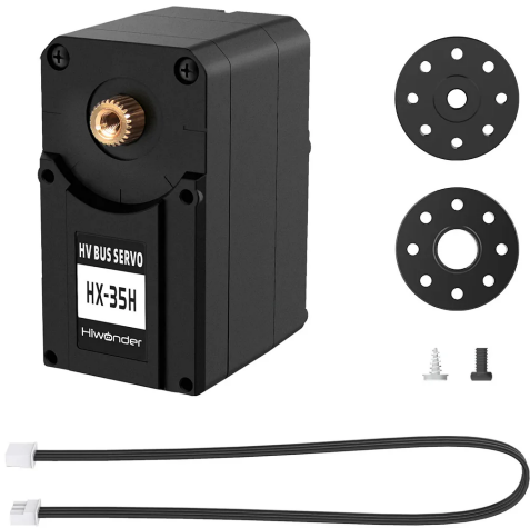
Figure A.2: HX-35H intelligent serial bus servo used in JetHexa joints
