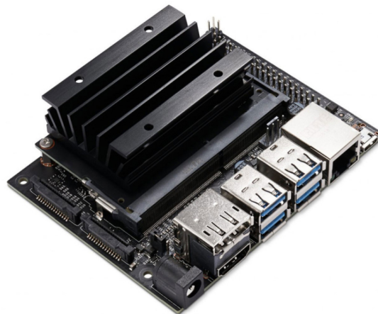
Figure A.3: NVIDIA Jetson Nano B01 development board integrated in JetHexa
