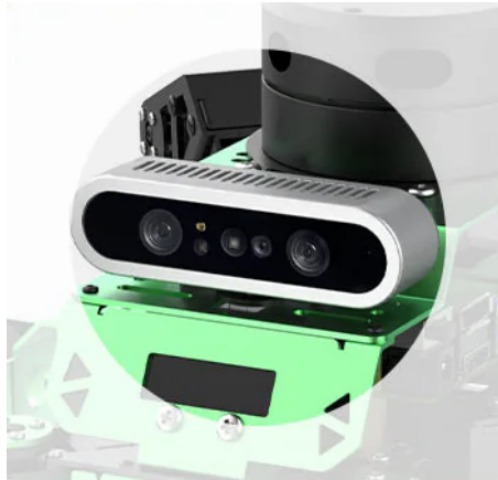
Figure A.5: 3D depth camera mounted on JetHexa for visual perception
