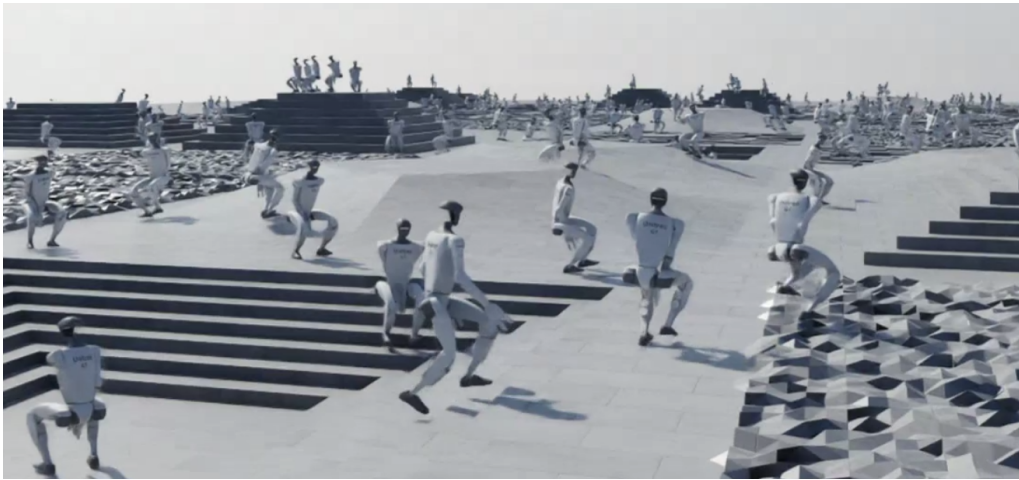
Figure 5.4: Parallel training of G1 robot following multiple movement commands
